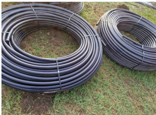
Standard 40 mm HDPE ducts and straight connectors
