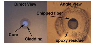
And remember to check that no power is present in the cable before you look at it in a microscope - protect your eyes!
