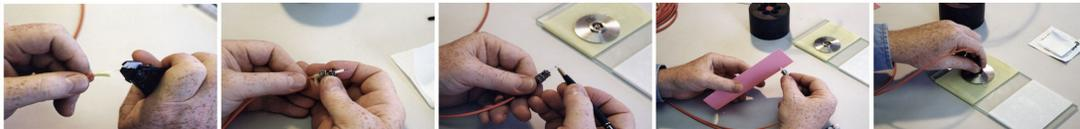
**Splice:** a permanent joint between two fibers
