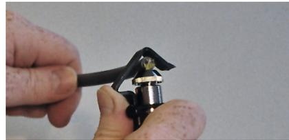
**Cleaver:** A tool that precisely "breaks" the fiber to produce a flat end for polishing or splicing.
