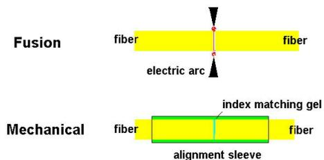
machines that do one fiber at a time or every fiber in a 12 fiber ribbon all at once. Good fusion splicers are expensive, but the splices only cost a few dollars each. Today's singlemode fusion splicers are automated and you have a hard time making a bad splice. The biggest application is singlemode fibers in outside plant installations.
