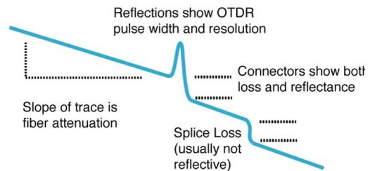
OTDRs can also detect problems in the cable caused during installation. If a fiber is broken, it will show up as the end of the fiber much shorter than the cable or a
