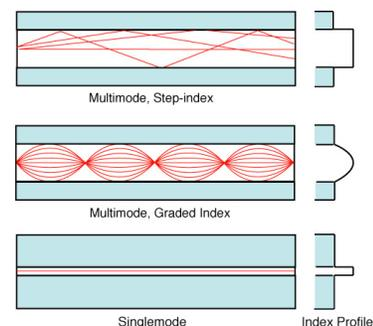
**Plastic optical fiber (POF):** is a large core (about 1mm) multimode fiber that can be used for short, low speed networks. POF is used in consumer HiFi and a new for car communication systems called MOST.
