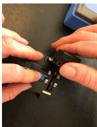
Open the top of the cleaver to expose the cleaved fiber - you may not see it is cleaved so don't trust your eyes
