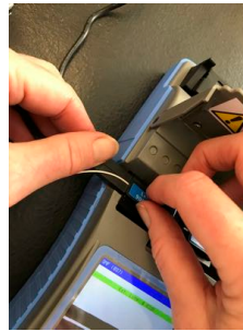
Open left fiber holder to release the fiber - don't stress fiber
