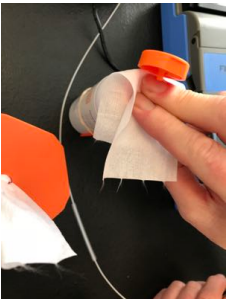
Wet a lint-free wipe with fiber cleaner
