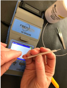
Slide heat-shrinking slice protector on fiber
