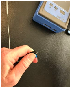
900 micron buffer is stripped
