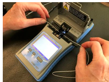
Gently lift both fibers out of the splicer - don't push toward each other or pull either
