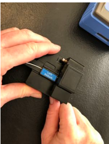
Push button on front of cleaver to cleave the fiber
