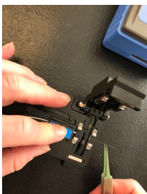
Remove the fiber scrap with tweezers or carefully with your fingers
