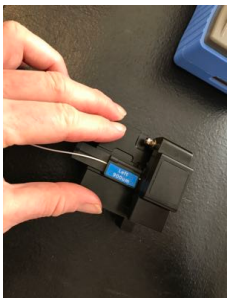
Close top of stripper gently - magnets will hold it
