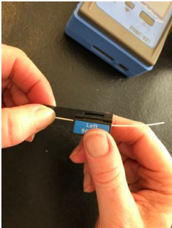
Make sure fiber is in groove
