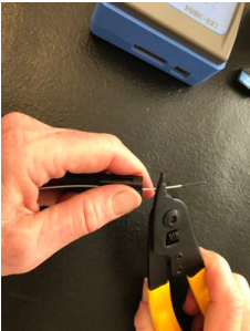
Second strip - note angle of stripper
