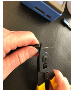
Third strip should be down to holder for minimum buffer.
