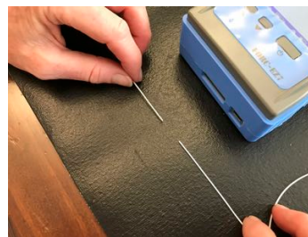
Lay fibers on work mat
