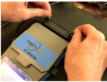
When heat cycle is over, open oven
