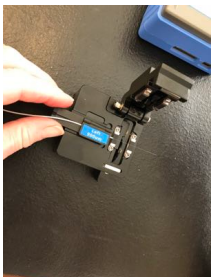
Place holder in cleaver - make sure it's fully seated in the slot and to the right
