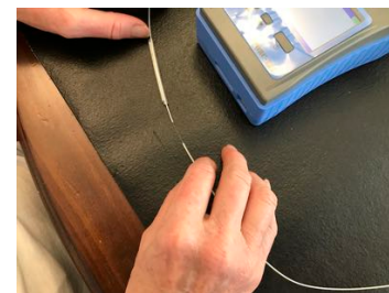
Slide heat shrink splice protector over splice - bare fibers should be in the middle
