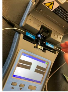
Insert the right holder and look for the second fiber in the display
