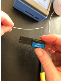
Place fiber in holder. If it is curled, align curl so it goes downward from top of holder
