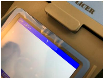
Display will show countdown - default is 60 seconds and works for usual protectors
