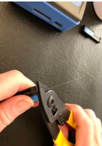
Gently strip 250 micron buffer with last groove on stripper jaws
